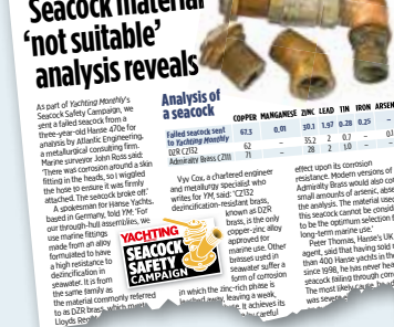
AUGUST 2011 YM sent a failed seacock from a three-year-old Hanse 470e for analysis. Severe electrolytic corrosion caused a through-hull fitting to fall off the outside of the hull of his 40ft ketch
