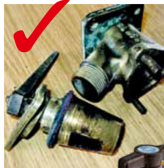
ABOVE: Blake's bronze seacocks are recommended RIGHT: Marelon plastic seacocks are increasingly popular
